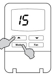
NOTE: The Installer Setup Menu settings are dynamic which means that nonapplicable settings will not be displayed. For example, if the thermostat is configured for heat only, settings not pertaining the heat only configuration will be hidden in the menu.
