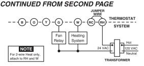
Figure 2. Typical wiring diagram for heat only, 3-wire, single transformer systems
