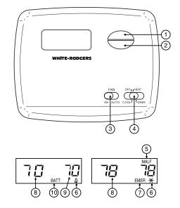
Figure 5. Thermostat display, buttons, and switches
