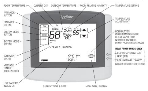
NOTE: BACKLIGHT IS ACTIVATED WITH FIRST BUTTON PRESS AND AUTOMATICALLY TURNS OFF.
