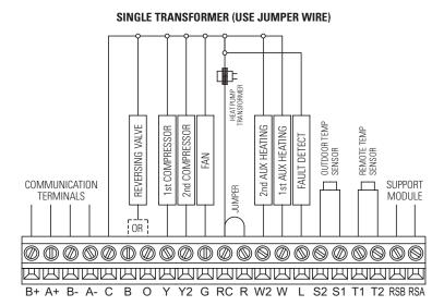
NOTE: "O" is active in cooling and "B" is active in heating.
