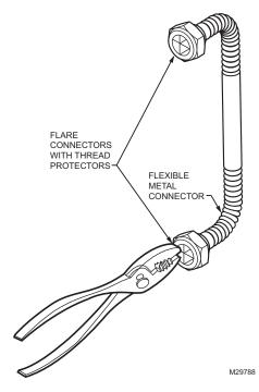
Fig. 4. Remove plastic thread protectors.
