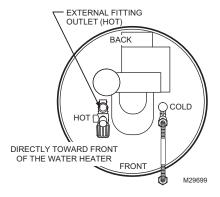
Fig. 6. Install mixing valve.
