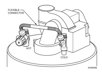
Fig. 7. Install flexible connector.
