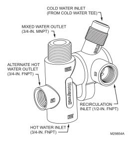
Fig. 2. Mixing valve connections.
