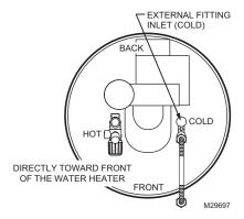
Fig. 5. Install cold water tee.
