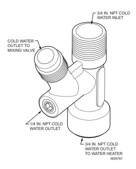
Fig. 3. Cold water tee connections.
