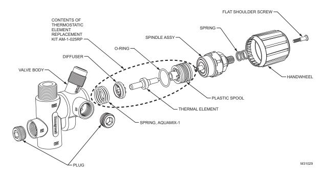
Fig. 10. Expanded view of AMX300 Mixing Valve.
