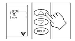
**Press** or to adjust the current setting. In AUTO use **MODE** to switch between the HEAT and COOL setting.
