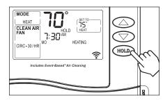
**Press** (HoLD) to permanently hold the temperature at its current setting. This will override the temperature settings for all time periods of the programmed schedule. With the thermostat in permanent hold, the thermostat temperature can be manually adjusted and will stay at that setting until the hold is cancelled.
