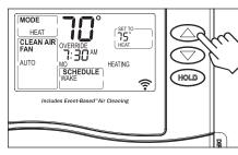
**Press** or to immediately adjust the temperature. This will temporarily override the temperature setting for the current programmed time period. The new temperature setting will be maintained until the next time period of the programmed schedule. To cancel the temporary override, **press** (NOLD) twice.
