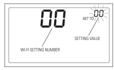
Press or to change the setting. Press MODE to change to the next option. Press MODE after the last setting. "DONE" will be displayed.
