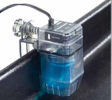
The CS1200 Multi-Position AC Shutoff Switch from DiversiTech is a reliable, easy to use float switch that clips on to any pan size. Designed with contractor feedback in mind, the CS1200 features an adjustable housing that twists to match any pan angle for easy installation. The CS1200 detects water in the pan quickly and shuts off the equipment to prevent damage. The CS1200 also includes these great features:
