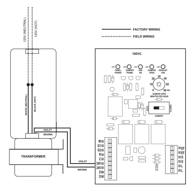
The iO-FAV-ENHANCED has a built-in 24 volt transformer used to power the outside air damper open when the panel calls for ventilation air.
