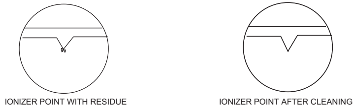
Fig. 19. Removal of deposits from ionization points.
