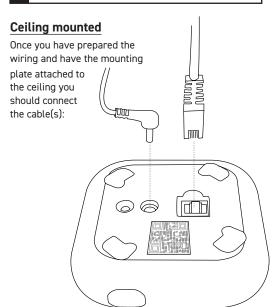
Then hook the FoobotSAT to the mounting plate and rotate it **clockwise**
