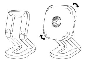
FoobotSAT and Stand can be placed on a desk, table, or furniture. Make sure to have to the user button located on the top right, so the monitoring sensors function properly. In this configuration motion detection will only cover a limited area.
