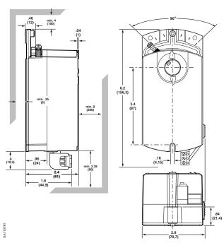
Figure 2. GDE Terminal Strip Model in Inches (mm).
