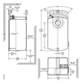
Figure 1. GDE/GLB Dimensions in Inches (mm).
