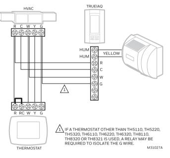
Fig. 8. Typical wiring diagram for humidifier using TrueIAQ.
