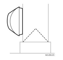
Fig. 2. HE360 Humidifier location in relation to air conditioning cooling coils.
