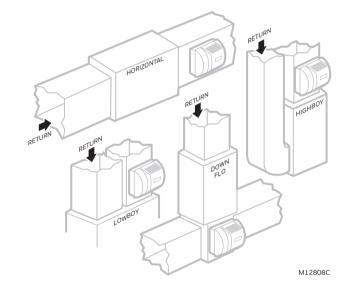
Fig. 1. Typical humidifier installation locations.
