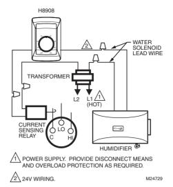
Fig. 3. Wiring diagram with H8908 (included) and current sensing relay (not included).\*
