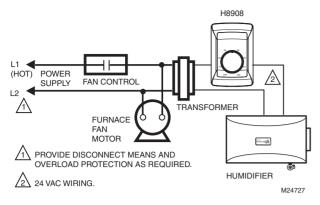
Fig. 1. Wiring diagram with H8908 (included). Transformer powered when single speed fan is energized.\*
