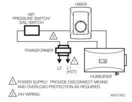
Fig. 4. Wiring diagram with H8908 (included) and sail switch (not included).\*
