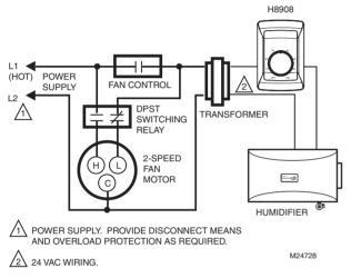
Fig. 2. Wiring diagram with H8908 (included). Transformer powered when two speed fan is energized.\*
