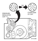
Fig. 1. Convertible Regulator for SmartValves.
