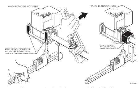
Fig. 5. Proper use of wrench on ignition system control with and without flanges.
