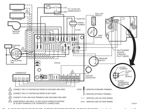
Fig. 9. SV9401/SV9402/SV9403, SV9501/SV9502/SV9503, SV9601/SV9602 typical wiring connections in fan assisted warm air furnace with electronic fan timer.
