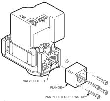
DO NOT USE FLANGES ON 3/4 IN. INLET AND 3/4 IN. OUTLET
