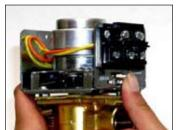
**NOTE:** The retaining spring presses on the outside of the bearing hub, but this does not lock the actuator in place. It is easy to remove the powerhead when the "Quick Fit" button is fully depressed.
