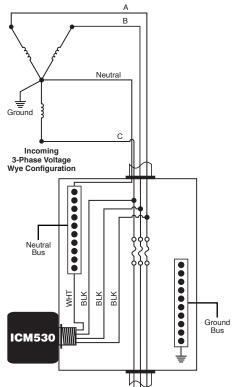
Type 2 Wiring - Circuit Breaker
