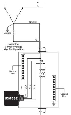
Type 2 Wiring - Circuit Breaker
