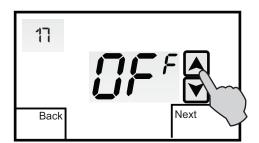
Adjustable from OFF, 32° to 122°F Remote outdoor sensor must be used
