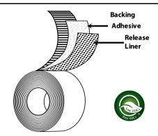
Printed 2.1 mil Aluminum Foil Backing:
