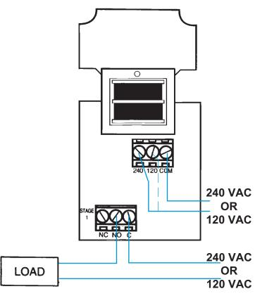
Figure 6: Different Voltage to Control and Different Voltage Load.
