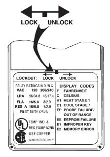
Figure 2: Lockout Switch
