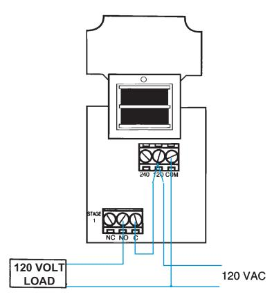
Figure 4: Typical Line Voltage Wiring Diagram.
