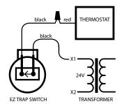
**Note:** Wiring diagram shown cuts power to thermostat when float switch operates to stop operation of the A/C unit. To inhibit mold growth during long absences, connect terminals into yellow cooling circuit so when float switch operates, condenser will switch off but fan will continue running.
