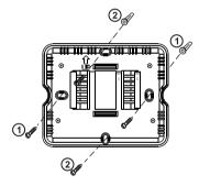
For a vertical mount, put screws on the top and bottom. For a horizontal mount, put screws
