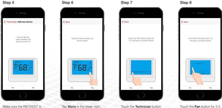
Touch the **Fan** button for 3-5 seconds, as shown.
