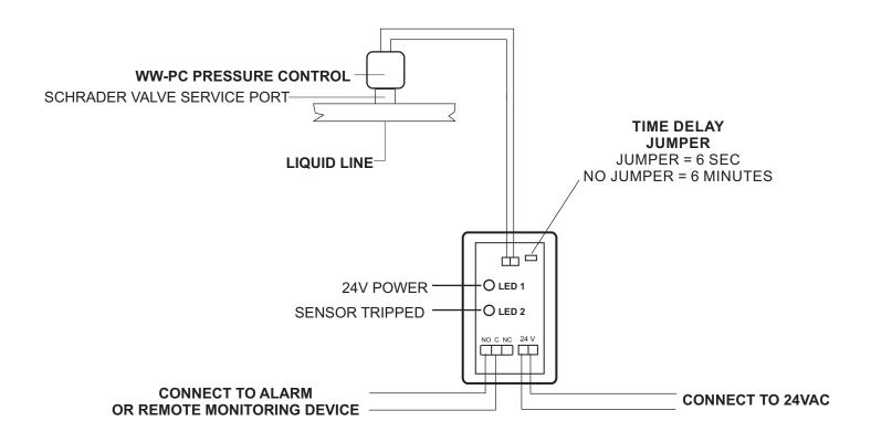
The UMM-RP can monitor refrigerant pressure using a pressure control mounted on the liquid line side of a compressor. If the refrigerant pressure drops below the setpoint of the pressure control, the relay contact can be used to trigger an alarm or remote monitoring device.
