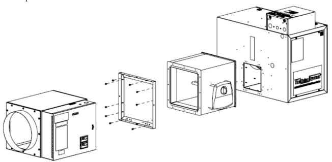
Figure 3. Installation of UV Cabinet with electric heater.
