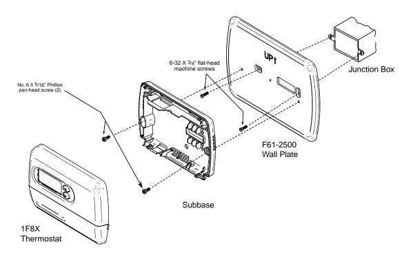
Figure 1. Mounting 1F8X digital thermostat to horizontal junction box
