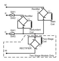
WIRING DIAGRAM - PILOTED MODELS 36H3X & 36H6X
