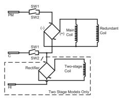
WIRING DIAGRAM - HSI MODELS 36H2X & 36H5X
