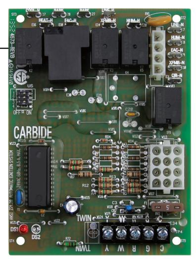
Integrated Furnace Module - 50A55-3797
