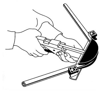
Easy one hand bending of 1/4" to 7/8" soft copper, aluminum and light wall hydraulic tubing. *Hard copper must be annealed before bending.*
