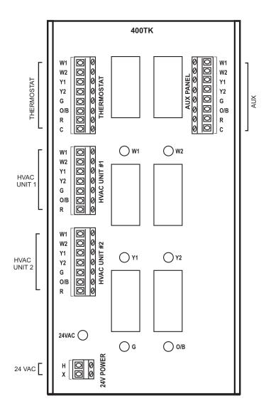
Wire appropriate HVAC unit to terminals marked HVAC UNIT #1 and HVAC UNIT #2.
