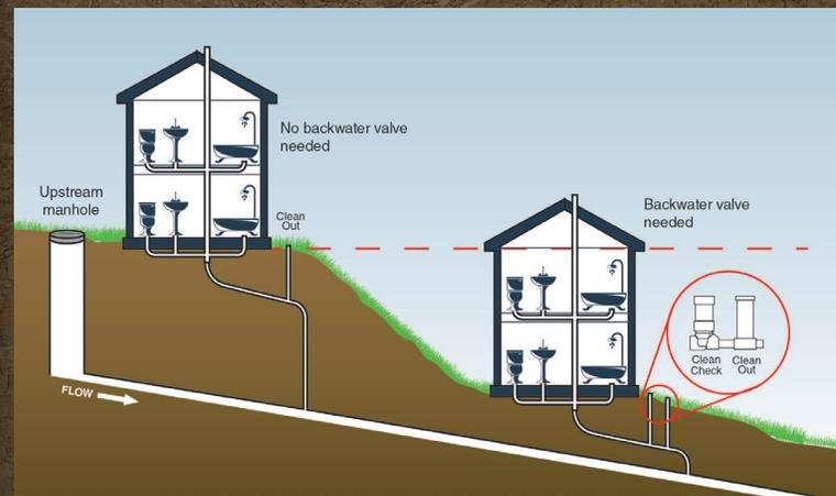
Waste water flow from structure. (Flapper opens)
