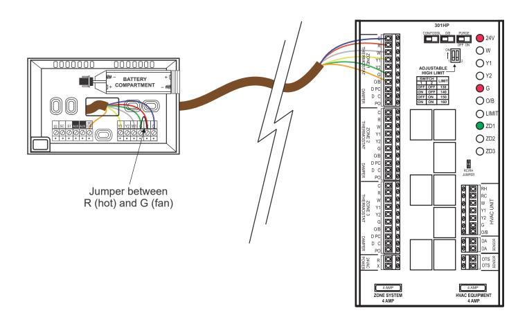
If there are voltage readings seen on the appropriate thermostat terminals, but there isn't the expected LED indication, confirm that there are not contradicting thermostat calls. Be sure the zone in question is the only thermostat making a heating or cooling call on the system.
