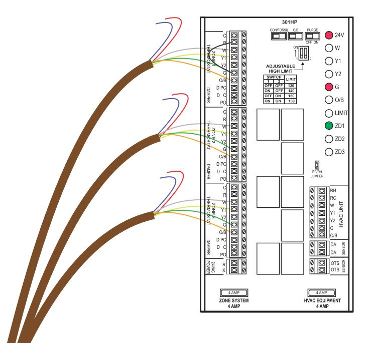
By inserting this jumper without power to the other zones, the G (fan) LED should light. If not, contact iO HVAC Controls for further tech support.
