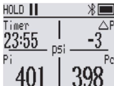
Figure 3 Pressure hold start interface
