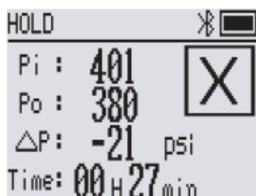
Figure 5 Test failure interface
