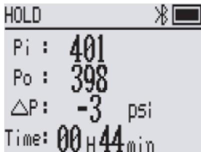
Figure 6 Test result display interface
