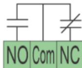
The Installer menu options will permit you to set this relay as a normally de-energised or as a fail-safe normally energised relay. This will change the NO/NC wiring logic.
