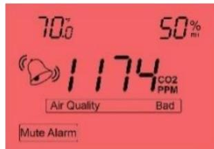
When enabled, user can mute an audible alarm by pressing the “Mute Alarm” button when shown. If Active Ventilation is enabled, the user can tap the “A” icon to briefly display the outside air temperature.
