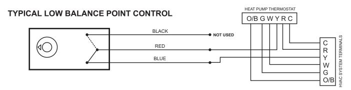
Used to prevent compressor from running when outdoor temperature is below a selected setpoint. Red and Blue open below setpoint.
