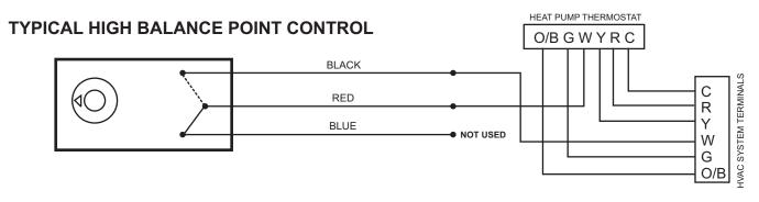
Used to prevent auxiliary heat from running when outdoor temperature is above a selected setpoint. Red and Black open above setpoint.
