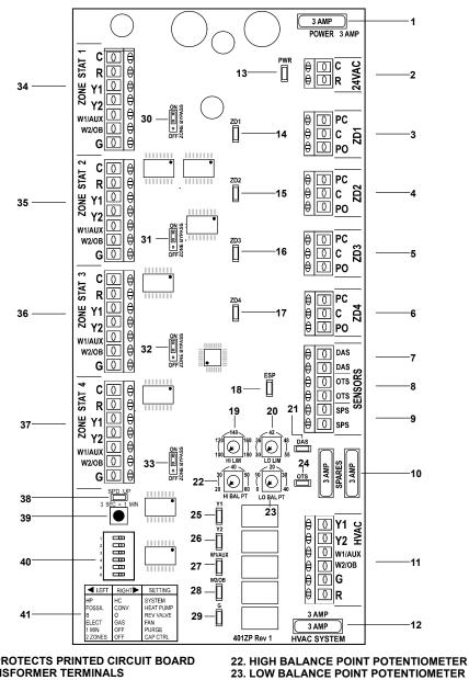
1. 3 AMP FUSE PROTECTS PRINTED CIRCUIT BOARD
