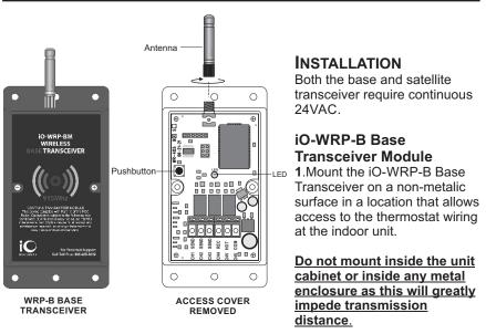
2. Once the base transceiver is mounted, take the access cover off by removing the two screws. Refer to the iO-WRP wiring diagram that best suits the application. Depending on the application, not all channels may be required.
