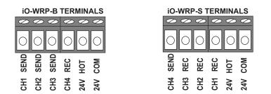
Please note the difference in terminal designations between the iO-WRP-B Base Module and the iO-WRP-S Satellite Module. The iO-WRP-B Base Module has three send and one receive channel. The iO-WRP-S Satellite Module has three receive and one send channel.
